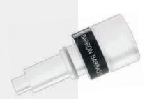
Two engraved ring reticles on the endpoint indicate a predetermined intraocular pressure of 65mm Hg or 90mm Hg. The smaller ring is 90mm Hg. The tonometer is 2.76 inches long and designed to be used with the Barron microkeratome. The 8mm contact tip is useful with small internal diameter microkeratomes.
