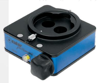
Designed to work with Zeiss, Zeiss type (Topcon, Moeller, etc.) and Leica (Wild) microscopes. Easy to operate with steam sterilizable knob. Short profile for use with all fixed and inclinable eyepieces. No light loss in upright mode. Virtually no image shift when switching between upright and inverting modes. Crystal clear optics. Compatible with all wide angle inverting vitrectomy lenses. Available with Ocular Wide Angle Vitrectomy Lenses.
